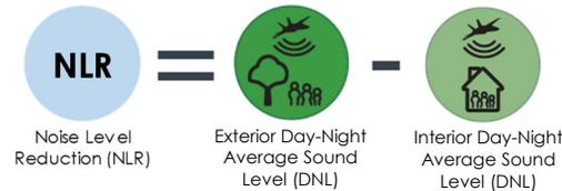
Sound travels from the exterior to the interior of a building by penetrating the building perimeter through the building's solid structural elements or via openings. Openings in the building (which provide air infiltration paths through windows, vents, and gaps) allow sound to travel directly into the building's interior. Basically, any place that air enters a home, sound will also enter.
